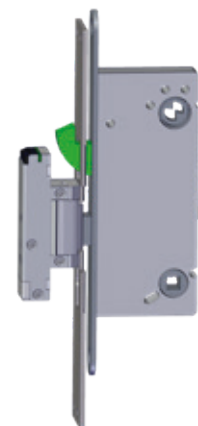
Here, a hook bolt is thrown through the faceplate into the electric strike's fixed cut-out and thus blocked the door's access control system/reader or door automation.
