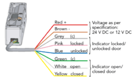
Wiring diagram with bolt contact.
