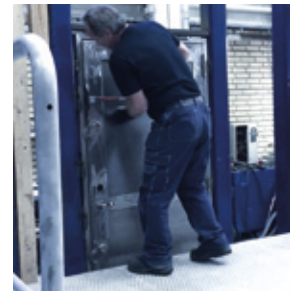
The picture shows STEP 18 Secure mounted together with Stålprofil in a sharp burglary test at RISE.
